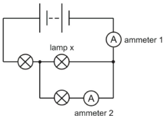
Lamp X 'blows' (the filament breaks). What happens to the reading on each ammeter, and to the total resistance of the circuit?
