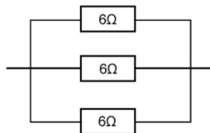
$$\begin{aligned} 1/\text{Total Resistance} &= 1/6 + 1/6 + 1/6 = 1/2 \\ \text{Total Resistance} &= 2\Omega \end{aligned}$$
