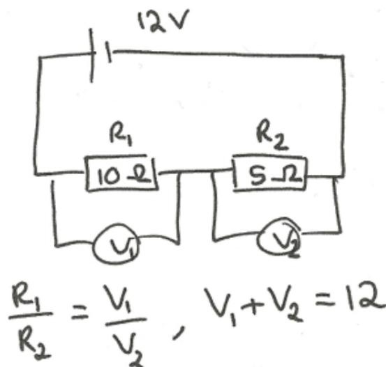
So, in this example, with resistors of 10Ω and 5Ω respectively, the maths is quite simple. The 10Ω resistor must have 8V going through it, while the 5Ω resistor has 4V. These numbers are easy (in that 10 is double 5, and splitting 12V into thirds is easy), but even with more difficult numbers, you should be able to do the calculations.
