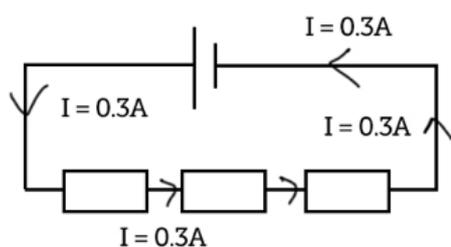
When drawing circuits, we represent current with a little arrow (as shown here). The arrow points in the direction of **conventional current**, which flows from **positive to negative**. Although electrons themselves flow from negative to positive, the convention was decided years before this was discovered, so when discussing currents, we say that **current flows from positive to negative** (The tall end of the cell is the positive end).
