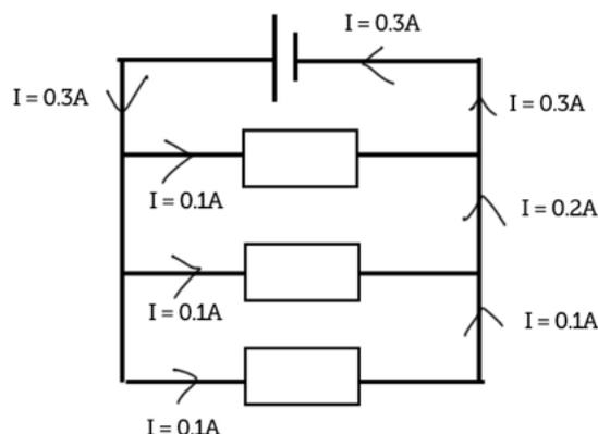
The  $0.3A$  current “splits” into 3 lots of  $0.1A$ , which rejoin to form  $0.3A$  towards the end of the circuit.
